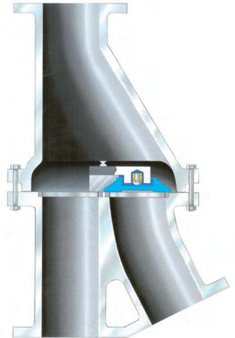
**THREE WAY, DIVERTING, OR CONVERGING.** This valve is shown in cast configuration suitable to 300 psig. Fabricated version is available for higher pressures and temperatures
