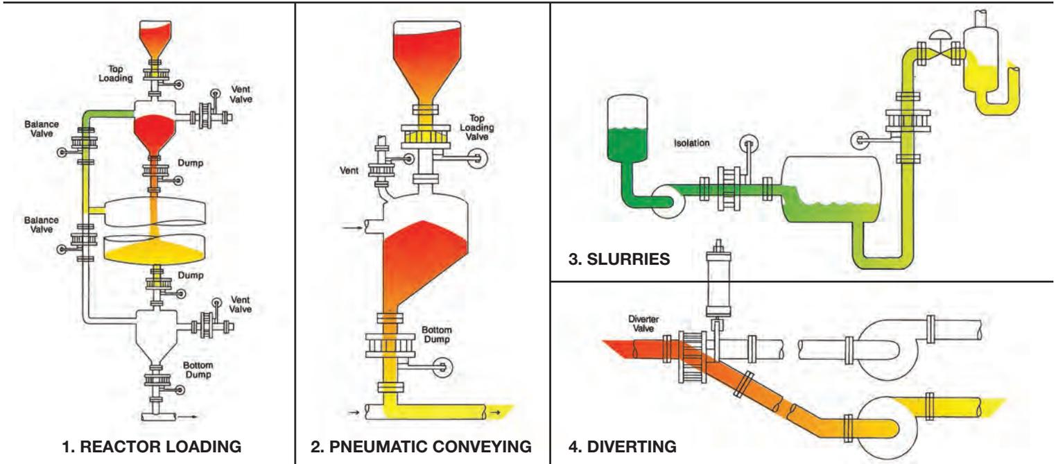
Their open body concept is self cleaning and incorporates precision flat lapped hard metal seals and discs that move in non-wedging, non-binding fashion through abrasive materials whether they are dry powders or in a slurry. Differences in tangential disc to seat friction cause the disc to rotate a few degrees with each cycle. This rotation polishes the mating surfaces improving the valve's seal with each operation. HERE ARE SOME APPLICATIONS
