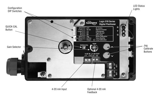
The Flowserve Logix 510si series are single-acting, user-friendly digital positioners. As with all positioners in the Logix 500si family, the Logix 510si uses the latest piezo-technology with inner-loop feedback to produce an improved dynamic behavior. The complete configuration can be made by DIP switches on the device. Different gain values allow the best setup for each individual actuator size.
