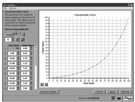
Figure 8: Manual Tuning with User Interface
