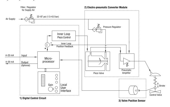
The Flowserve Logix 510si positioner is a digital positioner operated with an analog 4–20 mA input signal. The positioner consists of three main modules: 1) the microprocessor-based electronic control module with optional analog feedback and direct local user interface switches; 2) the piezo-valve-based electro-pneumatic converter module; and 3) the infinite resolution valve position sensor.
