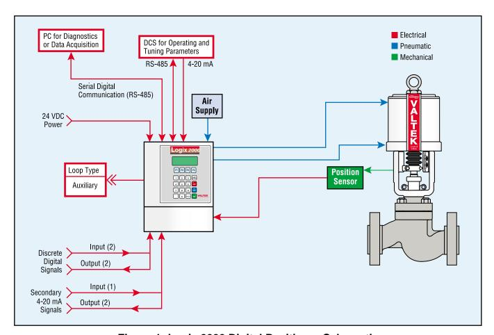
Figure 1: Logix 2000 Digital Positioner Schematic
