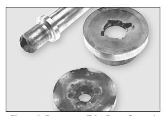
Figure 4: Damage to Trim Parts Caused by Cavitation
