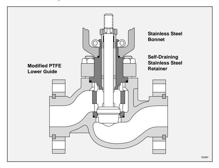
The Valtek® Mark One Sanitary Trim (Mark One-S<sup>TM</sup>) valve is a high performance control valve designed to meet the special requirements of the food processing industry. The internal parts of the valve are built with streamlined flow passages, eliminating pockets which could cause fluid stagnation.
