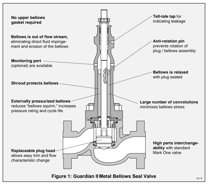
Wasted material, employee safety, environmental concerns and EPA regulations: all good reasons for today's plant operators to be concerned about fugitive emissions from hazardous processes. To stop packing leakage from control valves, Flowserve offers the Valtek<sup>®</sup> Guardian II<sup>™</sup> Metal Bellows Seal control valve.
