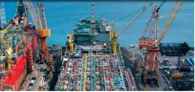
Offshore oil production facilities including over 50 wells, flow lines, risers, and two floating production, storage, and offloading vessels (FPSOs). Each FPSO produces 150,000 barrels per day and has a 2 million barrel storage capacity.
