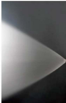
弹簧可调雾化喷嘴100%流量 Spring adjustable atomizer 100% flow
