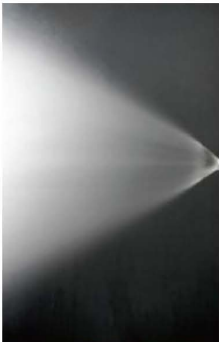
弹簧可调雾化喷嘴10%流量 Spring adjustable atomizer 10% flow
