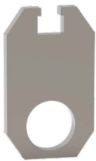
带导流孔闸板结构图 Structural drawing of RAM with diversion hole
