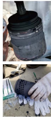
原调节阀阀芯磨损，套筒堵塞 The original regulating valve core is worn and the sleeve is blocked
